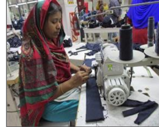
Photo of non-conformity Overlock operator not using mask and eye shield.JPG
