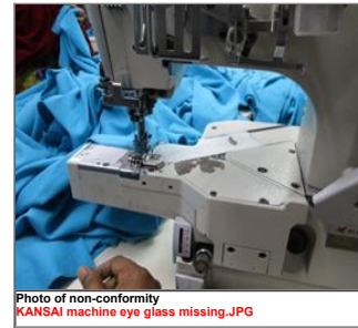
Photo of non-conformity Eye glass found missing in bertack machine.jpg
