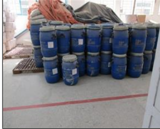
Photo of non-conformity Chemical drum kept without secondary containment.JPG
