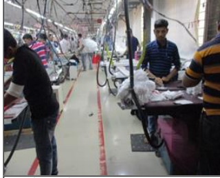
Photo of non-conformity 0.75 meter gap not maintained in the finishing pressing section.JPG
